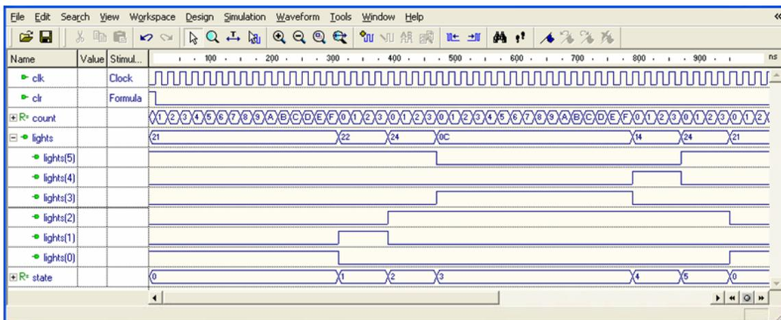
Figure 8.15 Simulation of the Verilog program in Listing 8.4
