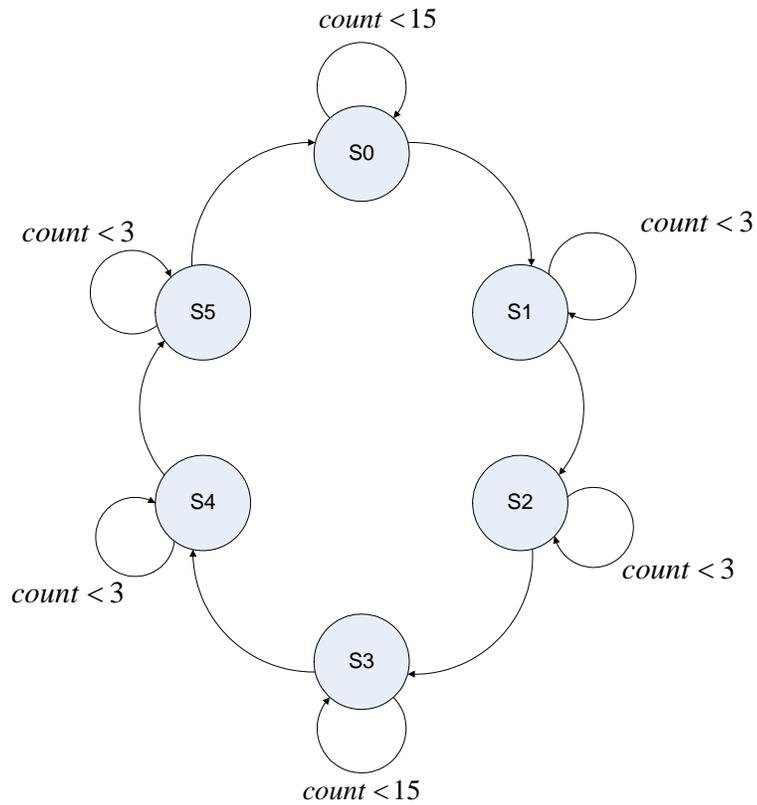
Figure 8.14 State diagram for controlling traffic lights
